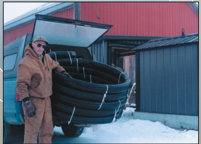
100 ft (33 m) x 4.9 in (125 mm) OD coil of dual PEX-Flex
